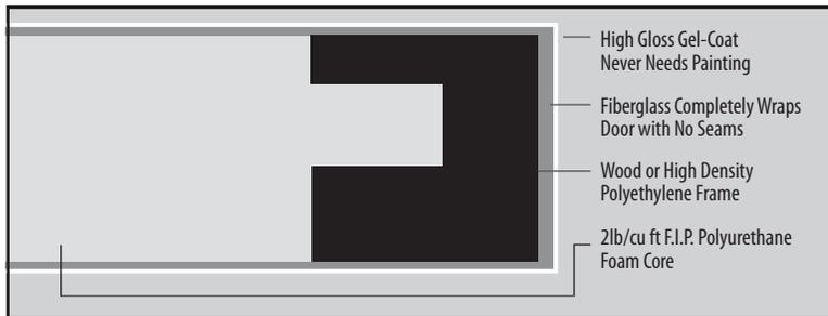
There is a major difference between fiberglass doors. Some manufacturers make their fiberglass doors by bonding together two shells and gel-coating to fill the seams. Other companies simply glue together panel surfaces and edges. These approaches may yield a nice looking door at first, but can leave the door susceptible to separating and delaminating when placed in abusive environments.
